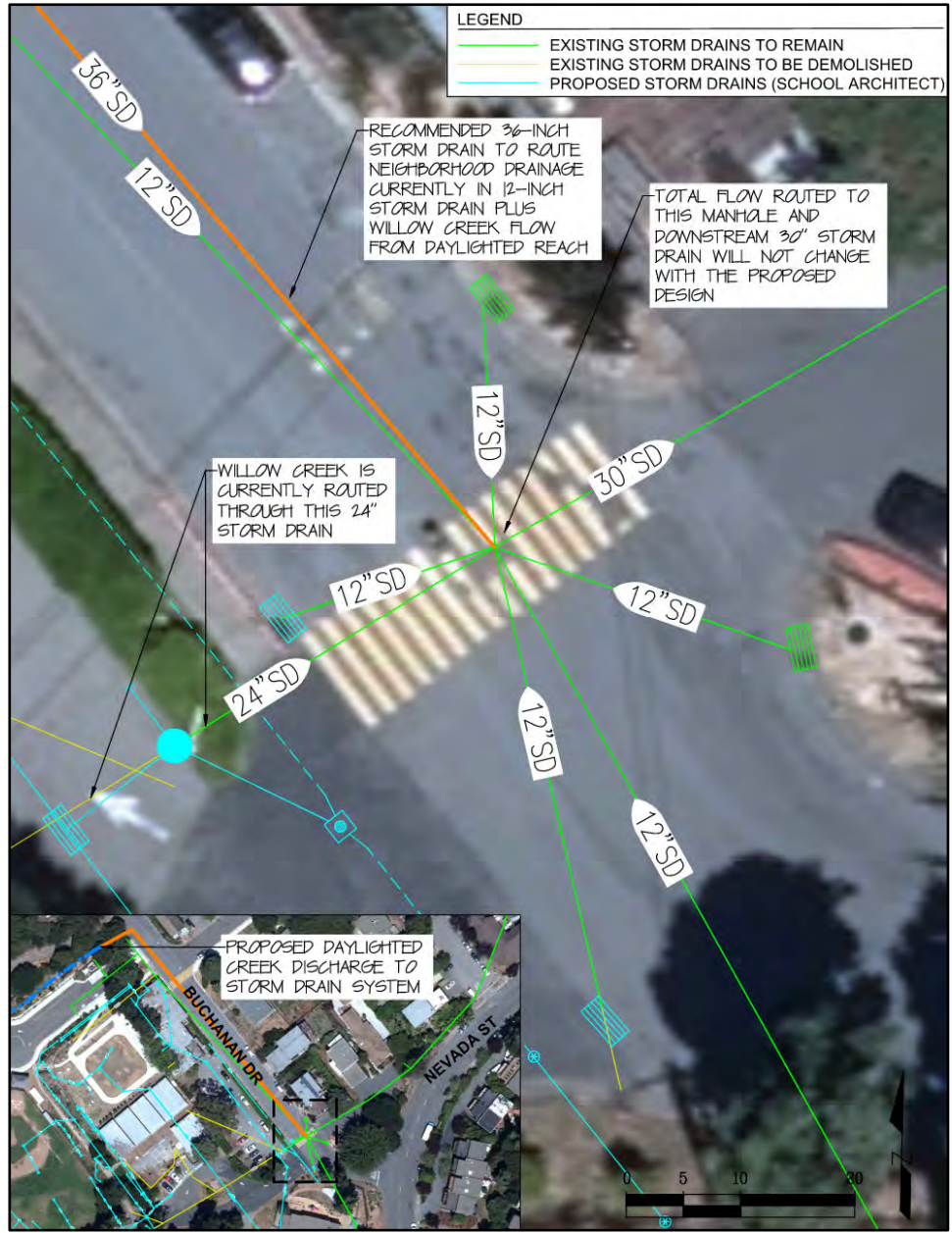
Figure 4: Existing and proposed storm drains at Buchanan Drive and Nevada Street. The manhole combines flow from one 24-inch pipe (Willow Creek) and six 12-inch pipes into one 30-inch pipe.
